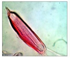
Fig. 1 : 123 x 29 µm extremely short vessels with circular perforation plate
