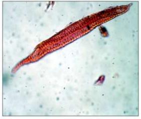
Fig. 6 : 162 x 16 µm Extremely small vessel
