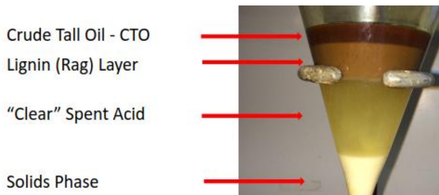
Figure 4. Phase separation of acidulated tall oil soap, as presented by Foran (2017).
