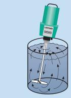
Angular Off-Center — Aiming the shaft off center prevents vortexing, and eliminates the need for tank baffles. Off center positioning achieves strong top to bottom turnover. Suitable for most mixing and blending.
