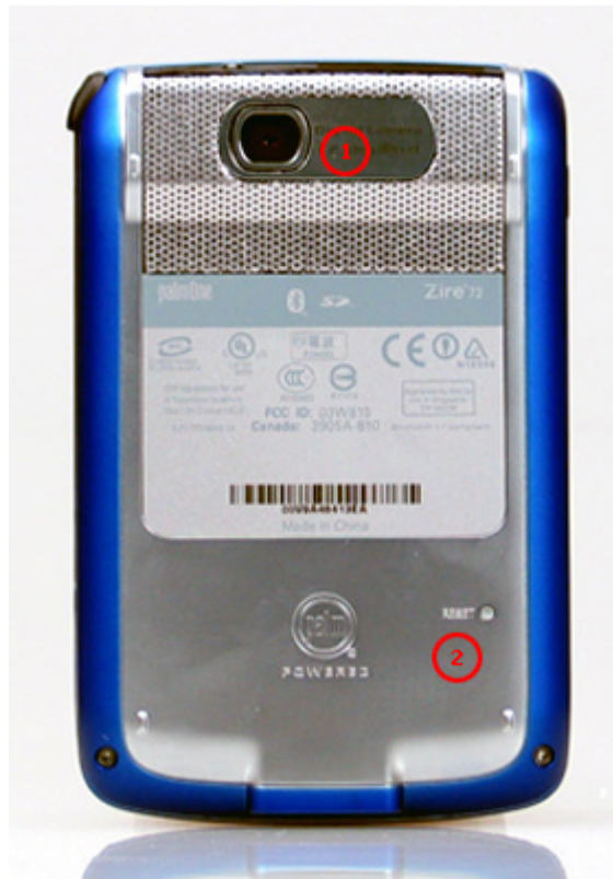
Rear View: 1. Built-in camera 2. Reset
