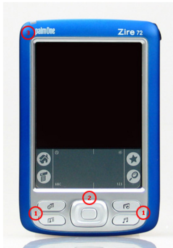
Front View: 1. Application/programmable button 2. 5-way Navigator 3. Power status
