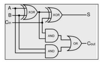
Here, there are 3 inputs & 2 outputs and 2 XOR gates, 2 AND gates & 1
