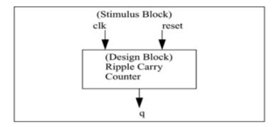
The second style of applying stimulus is to instantiate both the stimulus and design blocks in a top-level dummy module. The stimulus block interacts with
