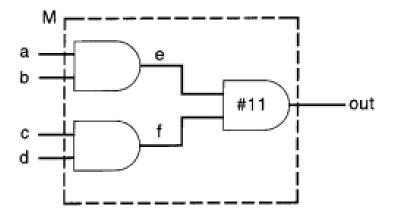
In this example we computed the maximum delay from any input to the output. The entire delay is lumped into the output gate. After a delay, primary output changes any input to the module M changes.
