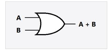
the OR gate has two inputs and one output. So the entity has totally 3 input and output signals.
