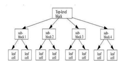
In this method, top-level block is defined and sub-blocks necessary to build the top-level block are identified. We further subdivide, sub-blocks until cells cannot be further divided, we call these cells as leaf cells.
