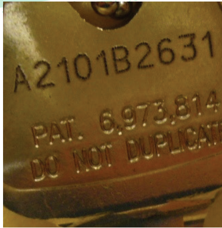
Figure 13. The Keso blind code on this key can be easily deciphered.
