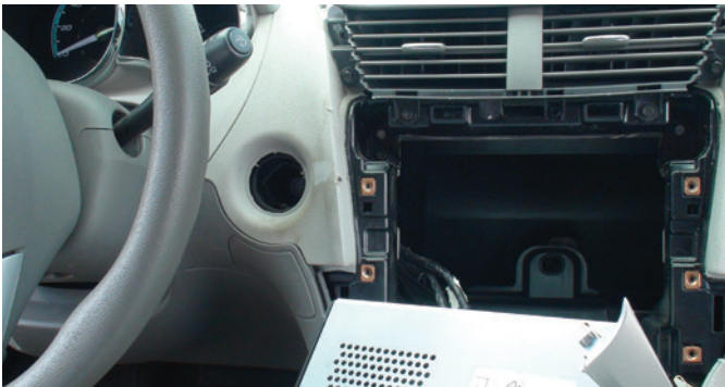
Figure 9. Then, remove the radio and the heater assembly to reveal the access hole to the retainer. See where the wires are coming out just above the radio? That is where you need to look for the access to the retainer.
