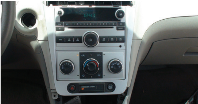
Figure 7. Next, you work the trim off from around the outside of the radio and heater controls. This trim is very tight, so be patient and work slowly.
