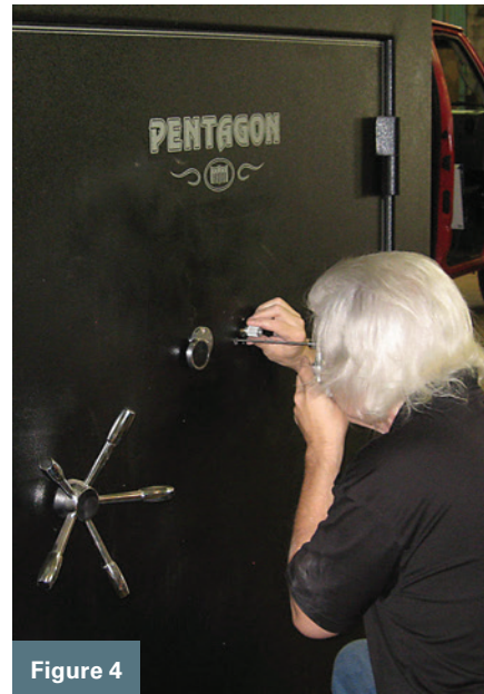
Figures 3 and 4. After a malfunctioning flex scope kept him from using the hole he had drilled in the side, the author ended up front drilling it and scoping the fence.
