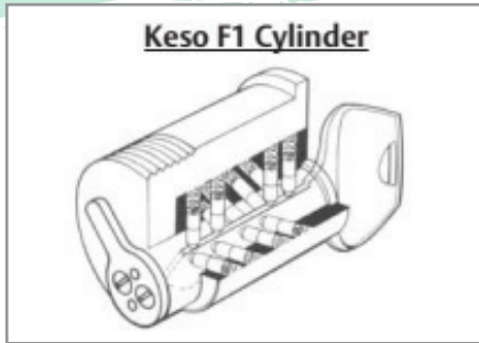
Figure 11. Shown is a cutaway drawing of the Keso F1 mortise cylinder, reinforcing the placement 12 chambers on three axes.
