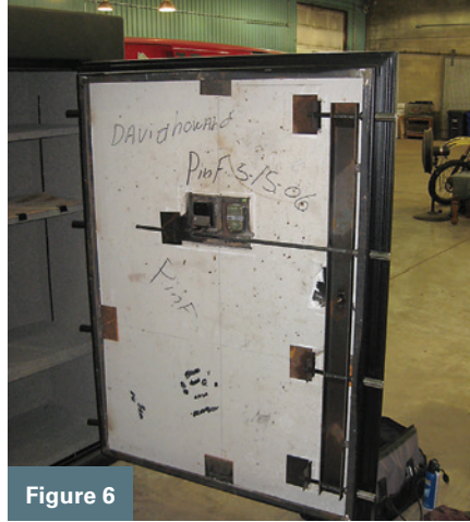
Figures 6 and 7. The locks are mounted side by side with only the lock on the right (from the outside) having a relocker.
