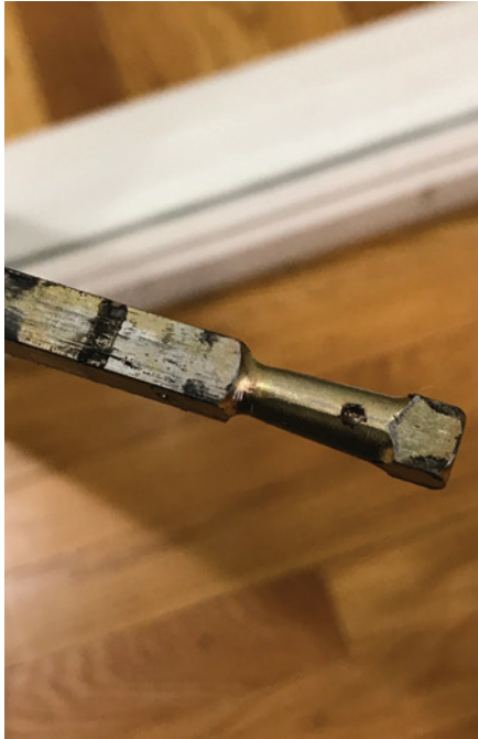
Figure 19. This image shows the indentation in the spindle made by the point of the set screw.
