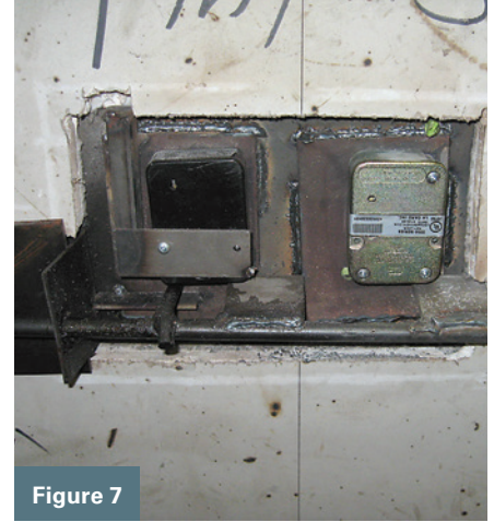
Figures 6 and 7. The locks are mounted side by side with only the lock on the right (from the outside) having a relocker.
