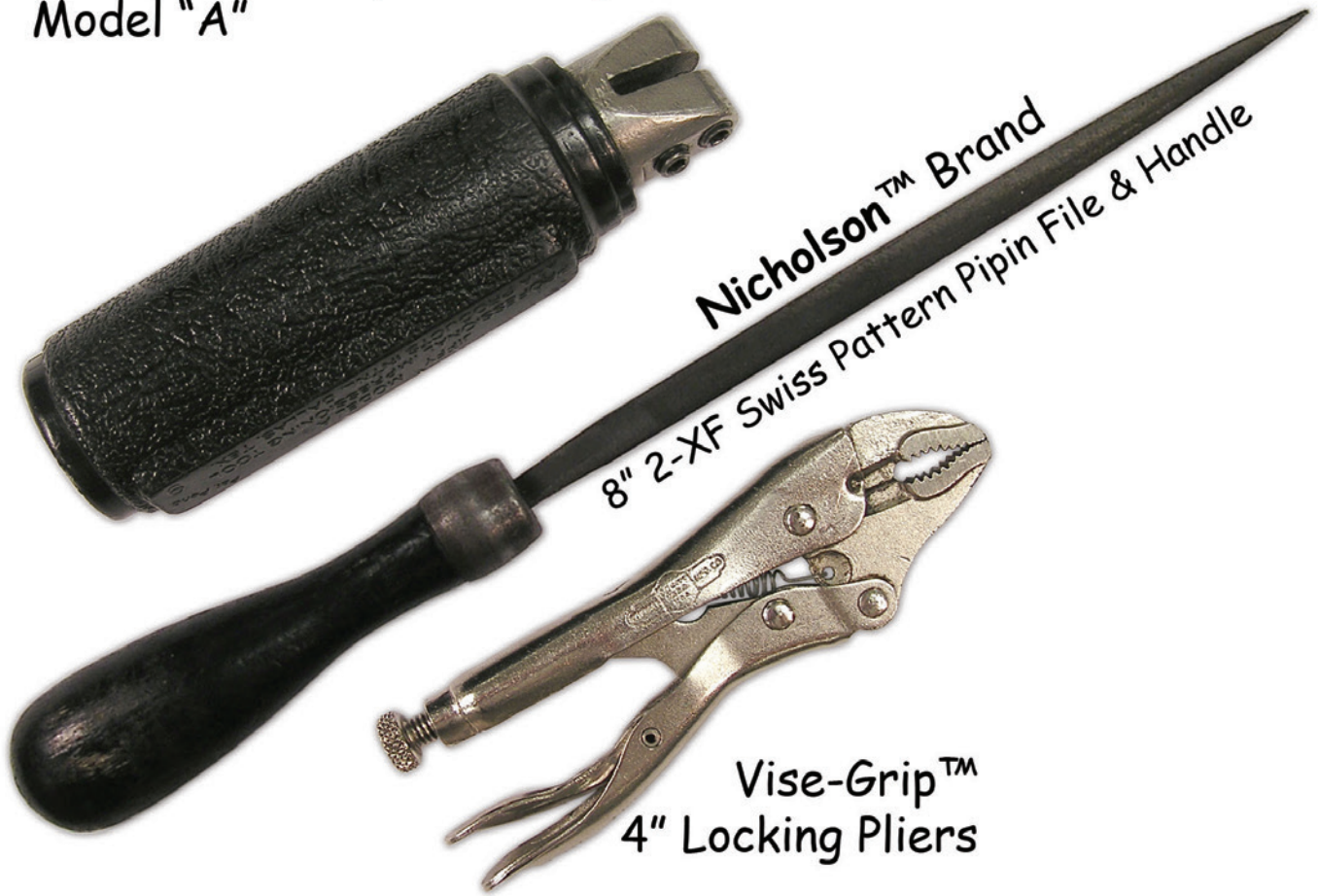
Figure 2. Two common tools used to hold keys for impressioning are the Jiffy Model A Professional Impressioning Tool and a common pair of Vise-Grip pliers.
