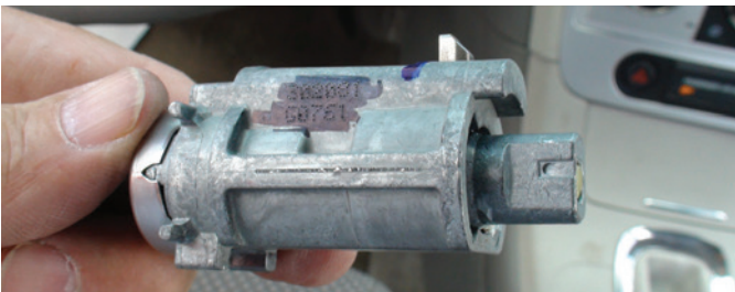
Figure 11. Fish around a bit, and you will feel it depress. You can then pull the cylinder out, and it will have a key code on it.
