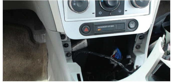
Figure 6. Once that is done, it will reveal two screws to take off.
