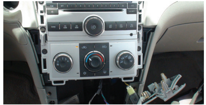
Figure 8. Once you get the trim around the radio and heater controls off, you will find six more screws to remove: two for the heater control and four for the radio.
