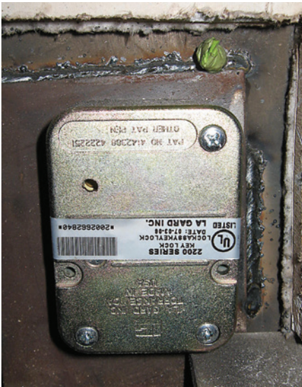
Figure 8. The hole at the top was “professionally” plugged.
