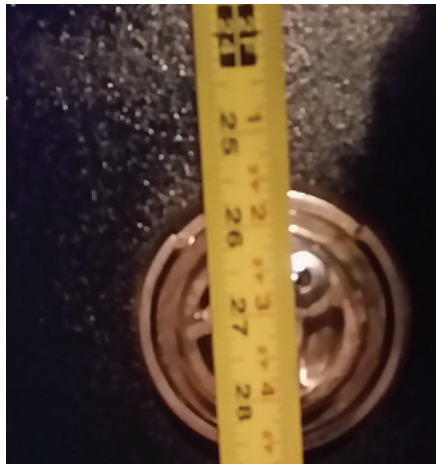
Figure 2. The measurement from the top of the safe to the center of the dial showed that the author's scopes were not long enough.
