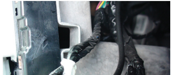
Figure 10. You will have to take a bent screwdriver or something similar, as you have a little bit of a bend to reach the retainer. But if you watch as you align it, you can find where the access point is. It helps to turn the key slightly back and forth so you will know by feel that you are in the correct place. The square hole here is where you go into the ignition. 🗝️
