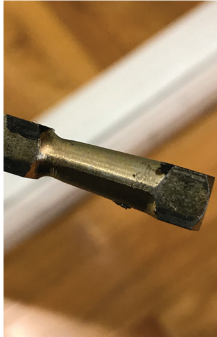
Figure 20. The author turned the spindle out a quarter turn to an unmarred surface before reinstalling the lever.
