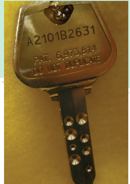
Figure 10. Pictured is an actual Sargent Keso change key with the eight dimple cuts shown on one side. Notice the depth differences.
