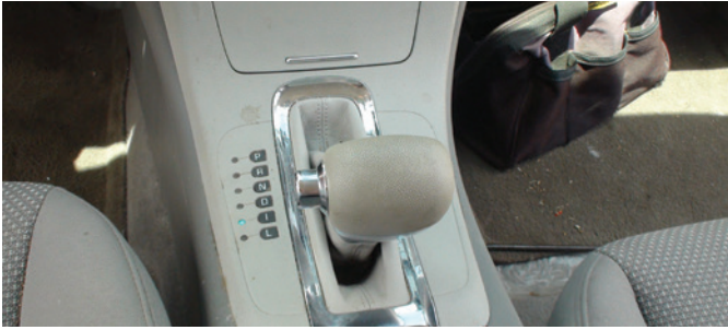
Figure 5. The plastic around the shift control will pop up so that you can turn it sideways to give you more room.
