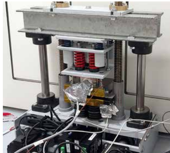
Apparatus for measuring force-response curves of cells due to swelling during operation [3]
