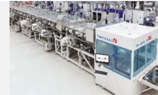
CSS Close Spaced Sublimation (CSS) for the Production of CdTe Solar Modules
